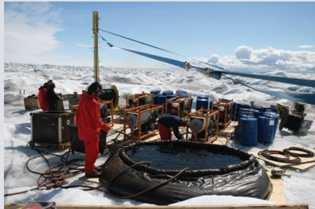
A hot water drill (supplied by AWI, Germany) in operation on Russell Glacier, Greenland, 2010. The black pool in front holds the water supply for the drill. The water is heated and compressed by the six heaters in the orange frames. The yellow winch in the background holds 650m of insulated drill hose which is guided down the yellow mast into the hole.
